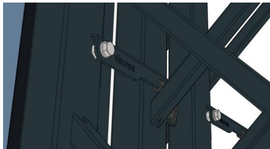
figure 9: Locking mechanism for gate elements
